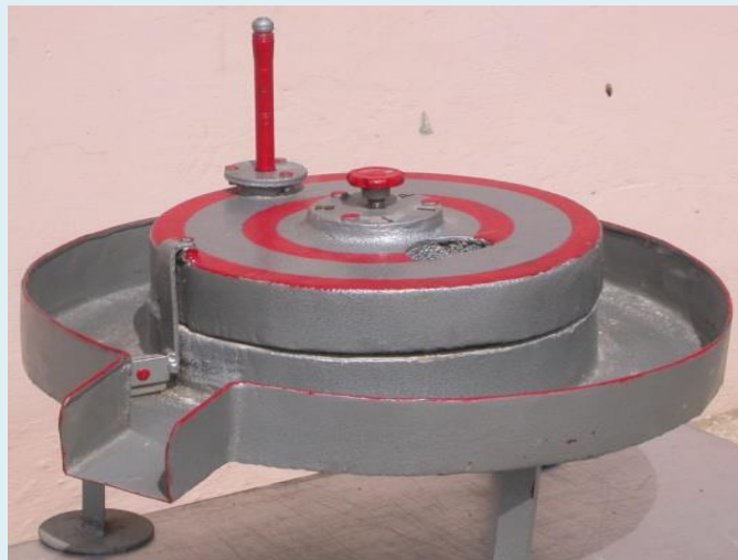
IIPR Hand Operated Horizontal Emery Dal Chakki
